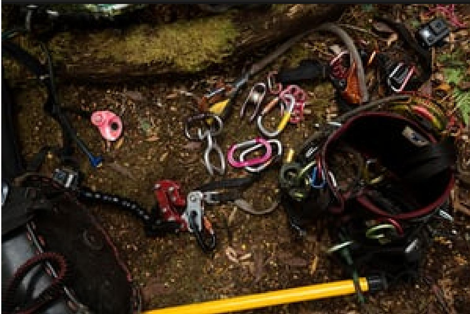
*Some of the climbing gear used to install and operate the camera suspension system. Along with camera equipment and personal climbing gear, more than 100kg of equipment had to be carried into the tree site.*
