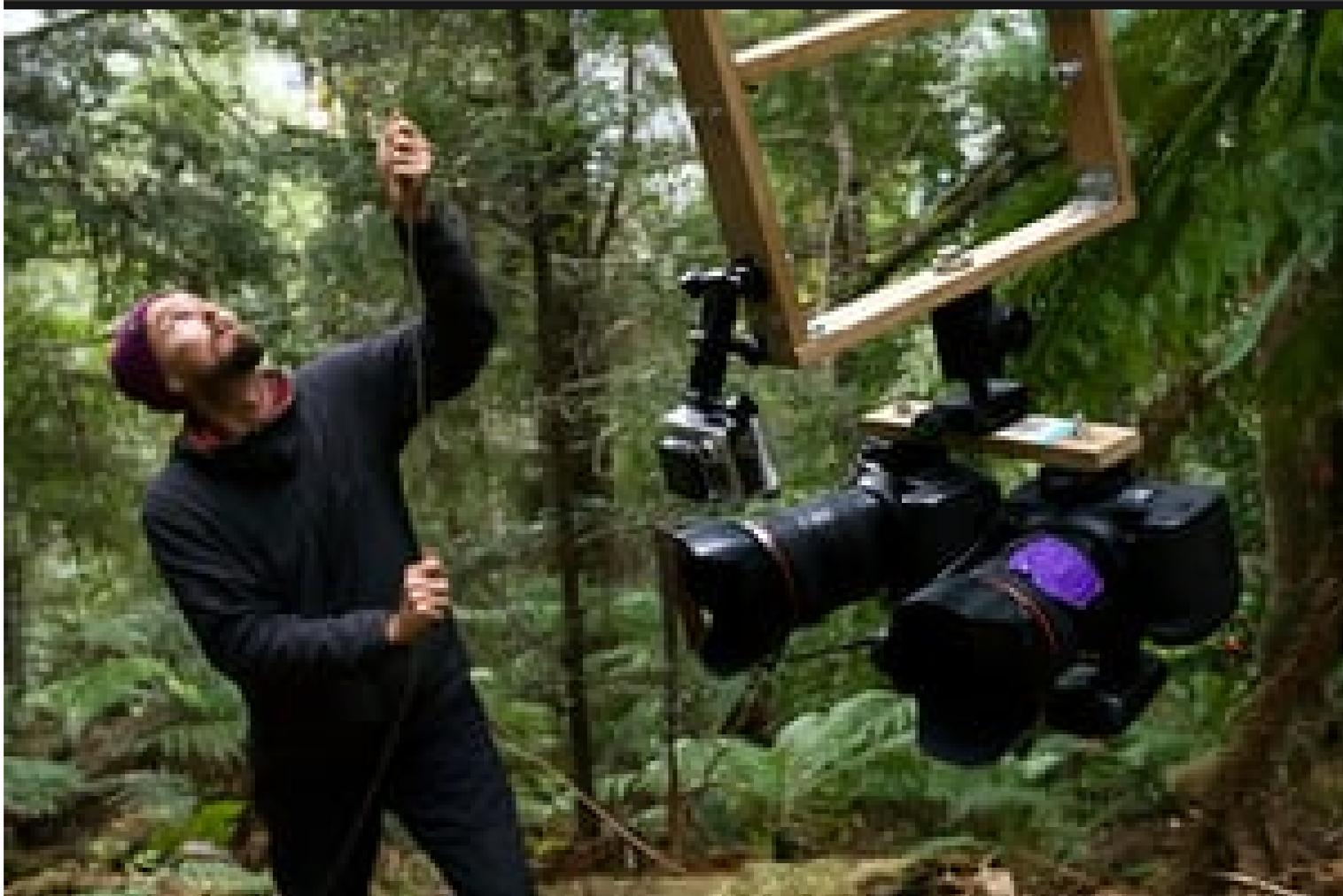
Photographer Steven Pearce checks and prepares to send his camera suspension system, affectionately known as MOE (margin of error), into the treetops. It was built from specialist climbing gear and items available from a hardware store. The main suspension rope was over 300m long and weighed 40kg.
